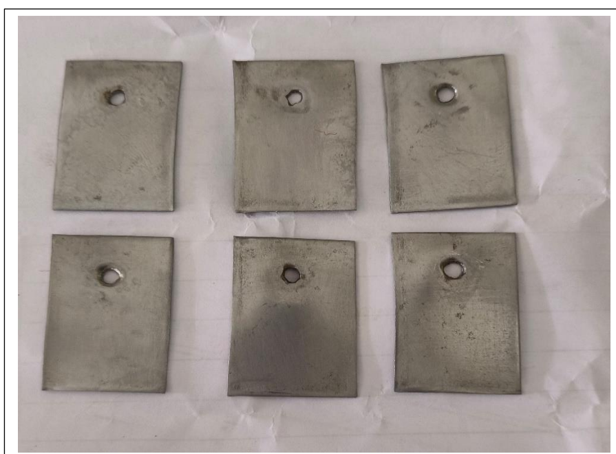
Figure 2.3: Mild steel sample for weight loss experiment
