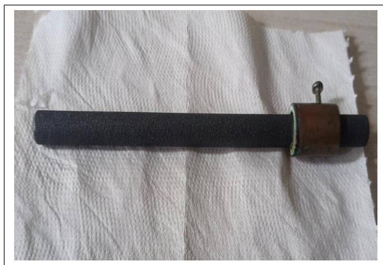
Figure 2.7: Graphite rod as Counter Electrode
