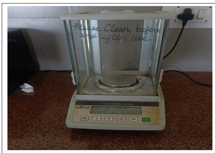
Figure 2.5: Weighing Balance used to weighing mild steel coupons
