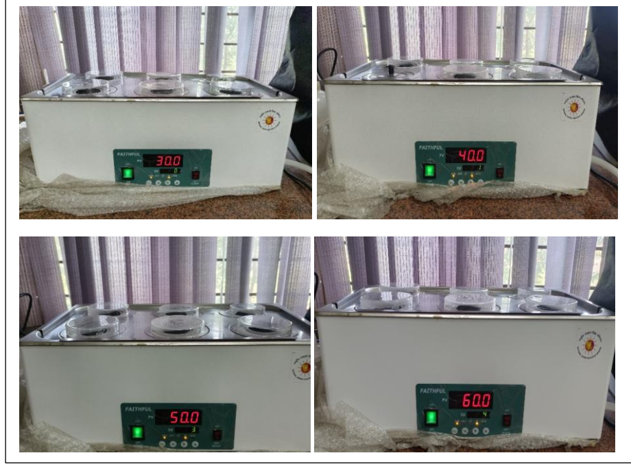
Figure 4.2: Gravimetric measurements (weight loss) in laboratory at different temperature (303 K, 313 K, 323 K, 333 K)
