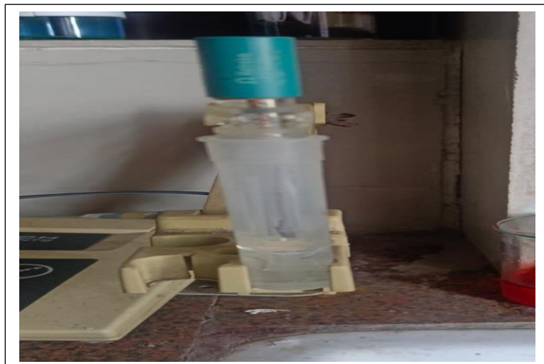
Figure: 2.8 Ag/AgCl(3MKCl) electrode as the Reference Electrode
