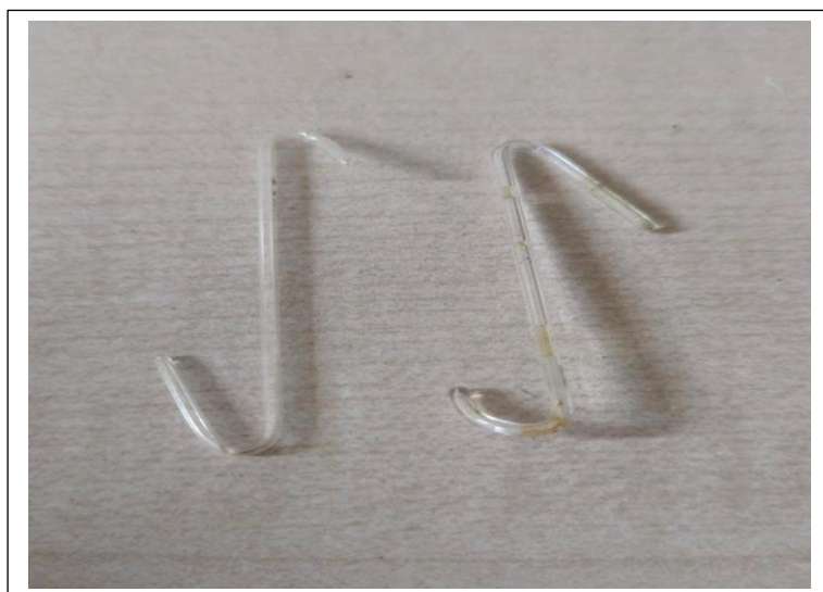
Figure 2.6: Glass hook used to hanging of mild steel coupon in corrosive solution
